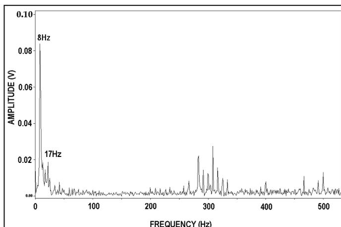
Figure 5: Frequency spectrum shaft misalignment at 500rpm.
